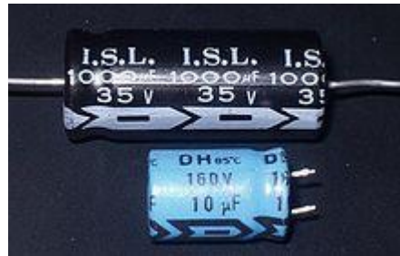
Fig. 2: Axial and Radial Electrolytic capacitors
